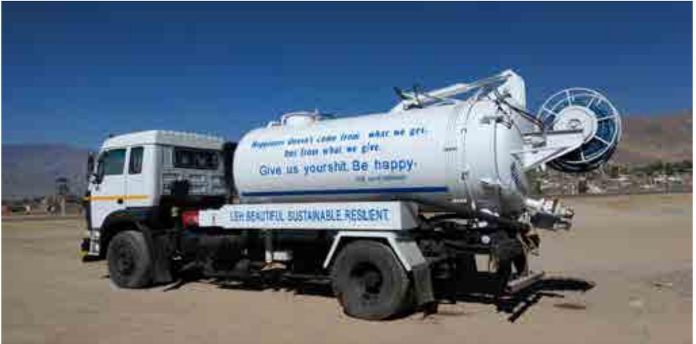
BWC developed a **double-booster pump mechanism** to overcome problem 1 and 2, by using off-board pumps in combination with the suction truck. This **innovation won the AMRUT Technology Challenge in 2018 from the Ministry of Housing and Urban Affairs (MoHUA)**, Government of India.
